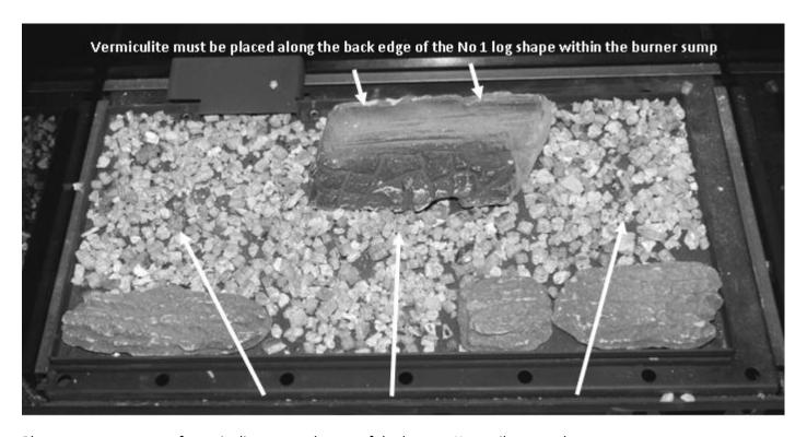
Place an even amount of vermiculite across the top of the burner. Keep pilot area clear.
