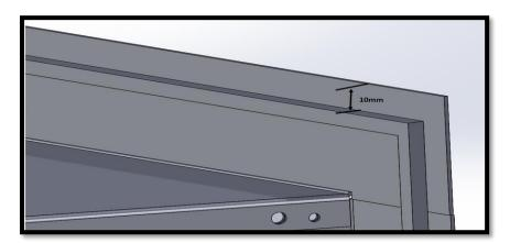
It is important to fit the installation seal leaving a 10mm gap between the top of the flange and the top face of the seal. (Please note failure to follow this guidance will not allow the fascia to be fixed correctly)
