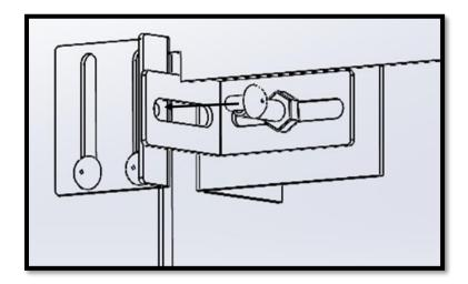
Fit the No6 screws to fix the fascia trim to the fire box assembly as shown in the picture opposite.
