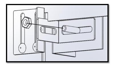
Below the fire tray assembly are two M4 stud left hand and right hand within the fire box assembly. Slide the adjustment brackets over the studs and fix using the M4 nut provided.
