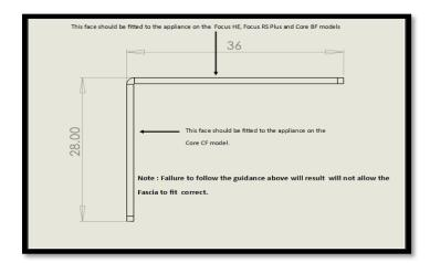
Within the fascia packaging are two adjustment brackets, two fixing screws and two M4 nuts. The adjustment brackets are design for use on various Paragon models. Please follow the instruction opposite to achieve the correct format for the model you are fitting.
