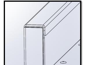
Offer the main frame up to the installed fire, slide the rear top edge of the fascia frame down in between the fire box flange and the fireplace back panel.
