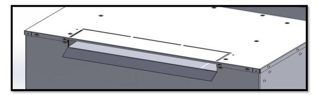
If the appliance is experiencing outing due to the flue having excessive flue draw, then the full restrictor may need to be fitted to combat this flue draw. This is provided in the box with the fire.
