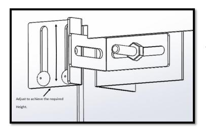
With the two adjustment brackets in position. Loosen the two screws holding the retaining bracket (on the main frame body) and move to the required height and tighten.
