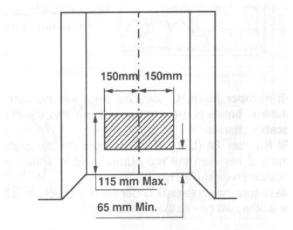
Drill holes for eye bolts on 112mm centre lines between maximum and minimum heights.
