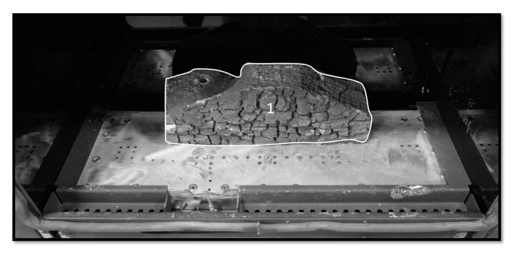
Place a thin layer of vermiculite over the burner as shown.
