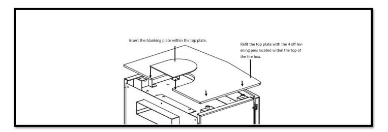
Note:- When installing the appliance using the above method. The appliance must sit hard against the closure place. This will allow 50mm of the rear spigot assembly to protrude into the catchment area.
