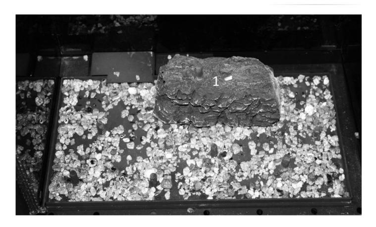
Spread a thin layer of vermiculite over the burner plaque taking great care around the pilot area.
