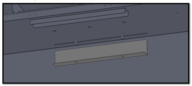
Please fit the 16mm restrictor plate provided with the appliance and repeat the spillage test procedure.
