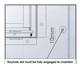
the 10mm clearance between the glass fixing bracket and the bottom internal edge of the
