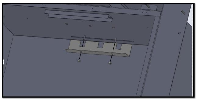
If spillage is still present after changing the restrictor plate you can remove it and repeat the test again. If spillage is still detected the cause must be discovered and the fault corrected. If the fault cannot be corrected, disconnect the fire from the gas supply and seek expert advice. Spillage can be caused by a restriction in the flue system, down draught, or insufficient ventilation into the room where the fire is installed.
